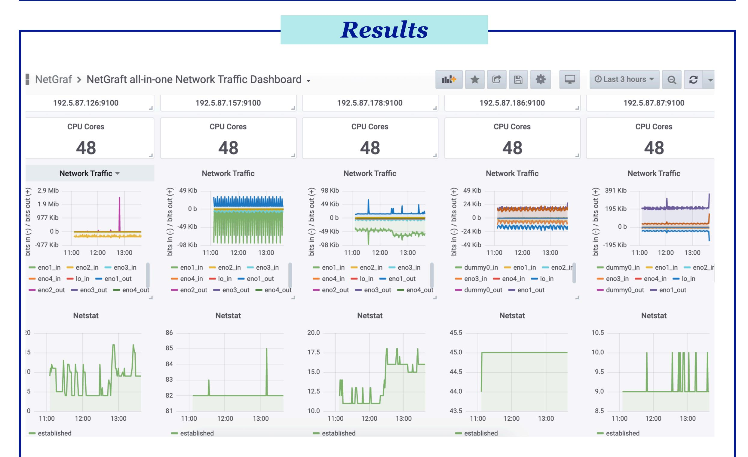
A snapshot of network metrics data collected, aggregated and visualized in real time in Grafana by five nodes from Chameleon testbed located at Chicago
